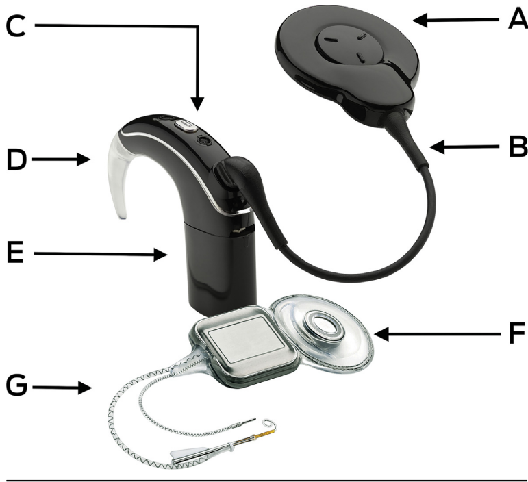
3 A current model cochlear implant. A. Transmitter. B. Transmitter coil. C. Microphone. D. Ear hook. E. Speech processor. F. Implant receiver/stimulator. G. Multichannel electrode array
