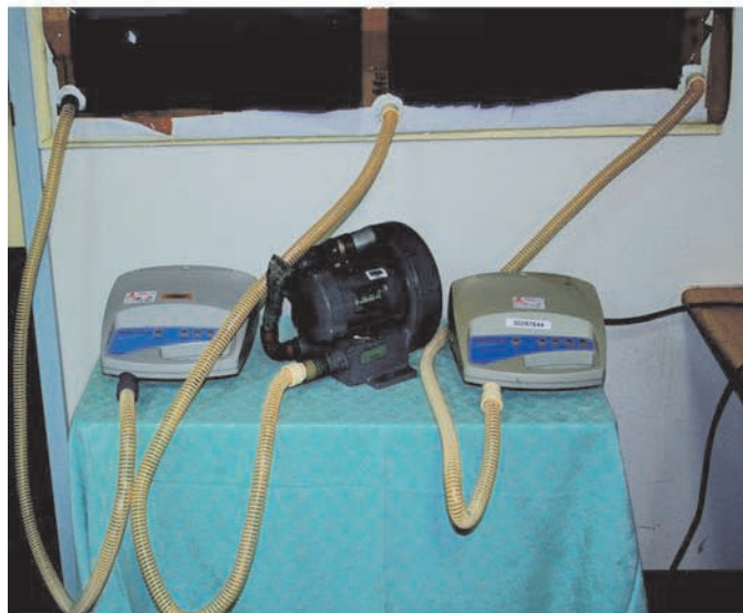
The three CPAP machines used to create the snow-dome effect. The Vortex blower is centre, with modern CPAP machines on either side.
